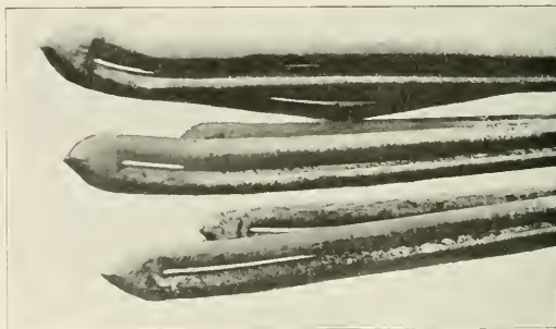
Distorted Ends of Superheater Units, One Result of Stopped-Up Flues
