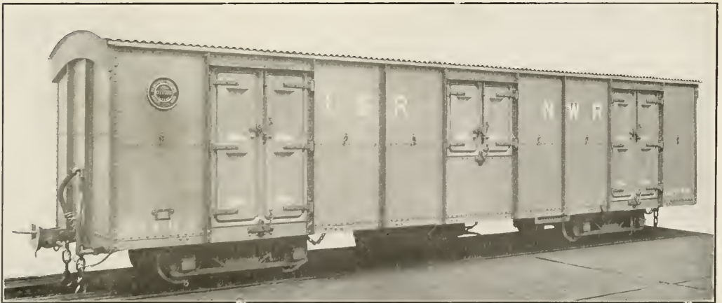
Box Car with Sheffield-Twinberrow Underframe and Trucks for the Kalka-Simla Railway
