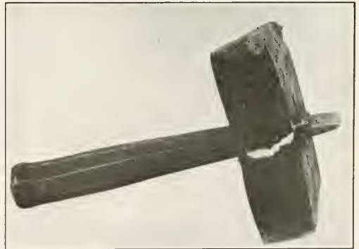
Fig. 2—A One-Inch Flat Chisel Driven Through 1 1/4-in. Stock
