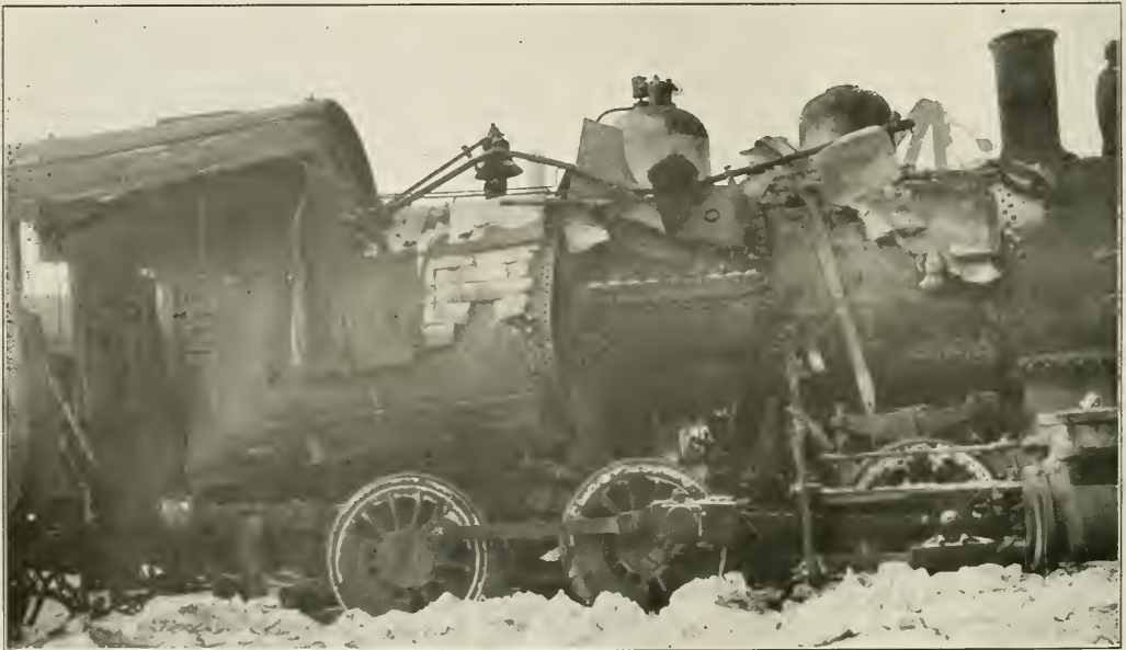
Wrapper Sheet Torn from Barrel Due to Low Water
