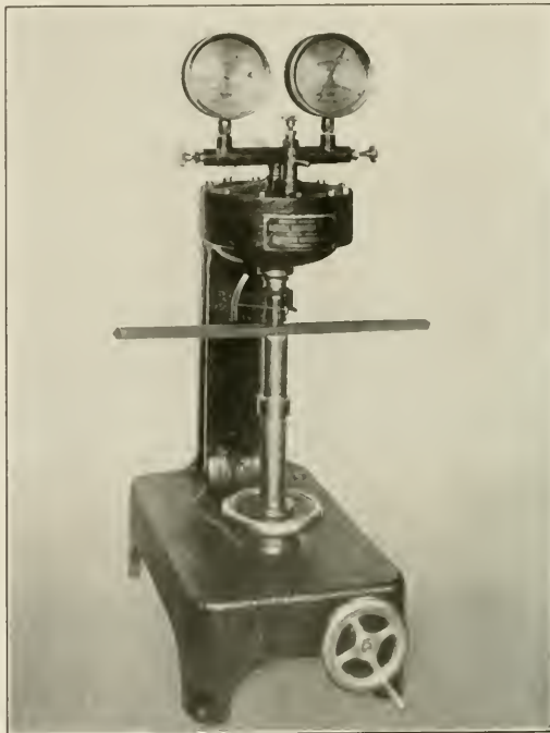
Fig. 3—Brinell Instrument Used in Testing the Hardness of Reclaimed Bars
