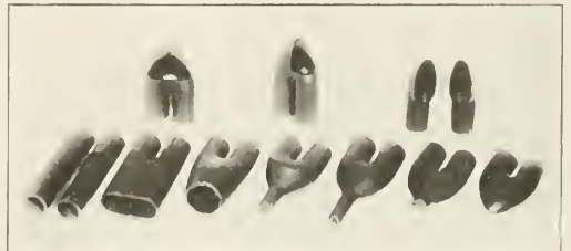
Steps in Forming Forged Return Bends in Superheater Units
