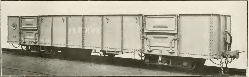
Narrow Gage Gondola Car of the Sheffield-Twinberrow Type for the Kalka-Simla Railway, India
