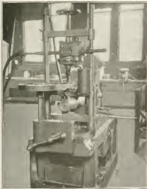
Milling Slots for Crosshead Keys in Special Machine
