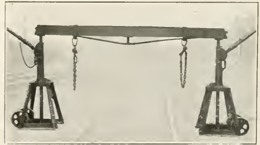
Fig. 2—Arrangement of Jacks for Use in Changing Truck Wheels
