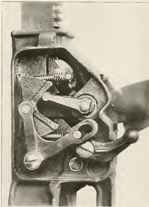
Operating Mechanism of Barrett Car Jack
