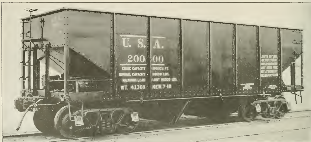
The First Standard 55-Ton Hopper Car to be Completed for the United States Railroad Administration Just Delivered by the American Car & Foundry Company; These Cars Will be Lettered with the Name of the Railroad to Which They Are Assigned
