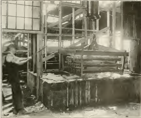
Fig. 3—Dipping the Axles in the Cooling Tank
