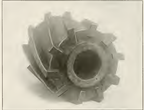
Fig. 2—Reamer Blades Inserted in Wax and Ready for the Mould
