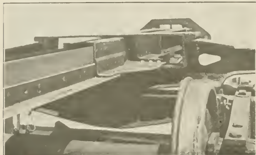
Draft Arm and Bolster Used With Girder Beam Underframe
