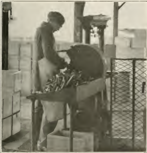
Fig. 11—Sharpening Track Spikes
