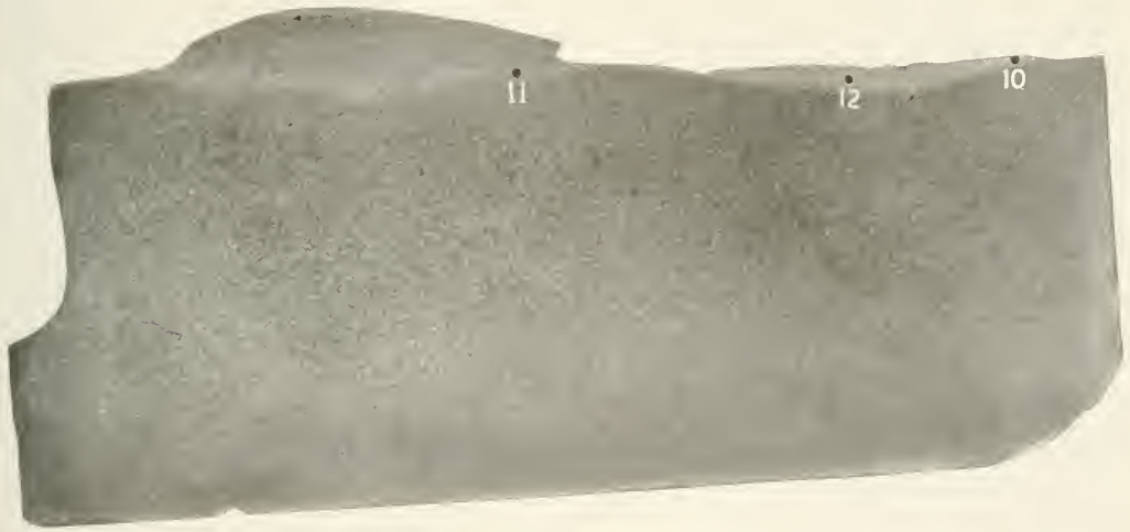
Fig. 31—Structure of Test Piece After Being Heated to the Melting Point—3.5 Diameter
