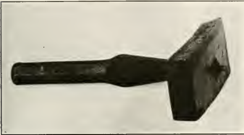
Fig. 1—A 5/16-in. Cape Chisel Driven Through 3/4-in. Stock
