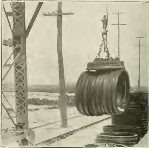
Electric Magnet Holding Tires—15,000 lb. Total Weight on Crane Hook
