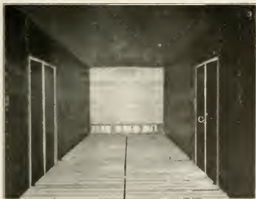
Completed Interior of the Car with the Usual Type of Floor Rack
