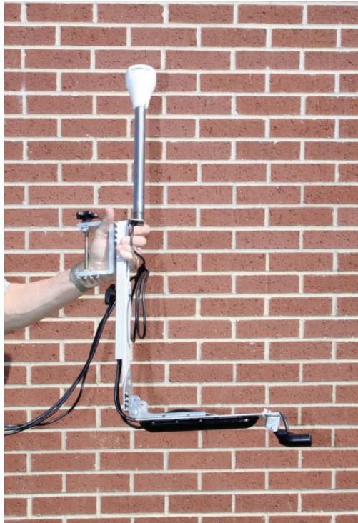
Figure A5. Transducers, mounted on pivot arm, and GPS antenna mounting bracket.
