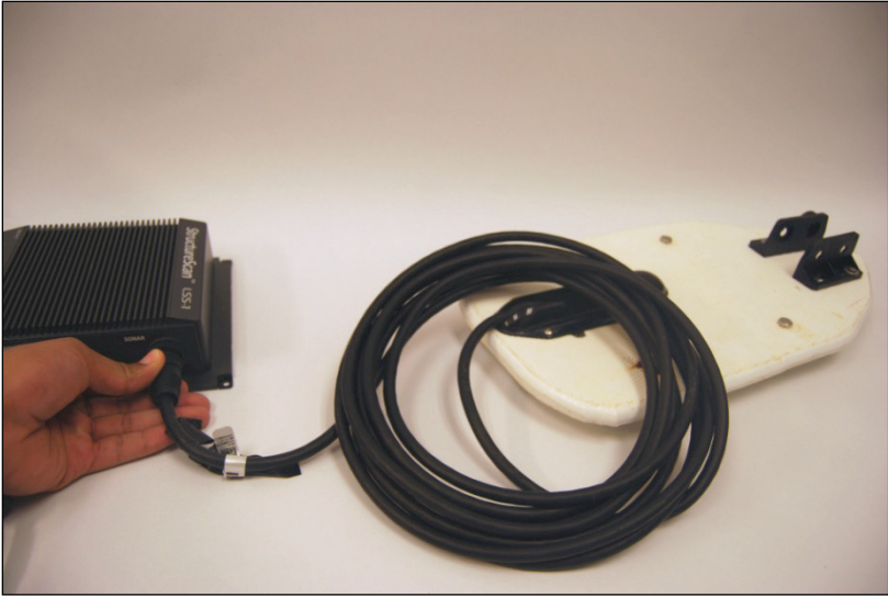
Figure 8. Structure Scan transducer cabling.
