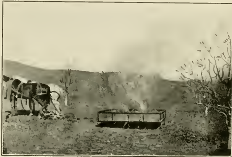
FIG. 193—PORTABLE BRUSH INCINERATOR Built of sheet iron on runners. Holes in the bottom admit air and allow ashes to fall out.
