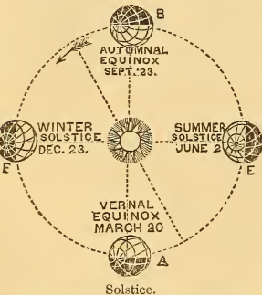
A and B, equal day and night; E, longest day, or summer solstice; F, shortest day, or winter solstice.
