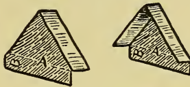
Cut "waste" away to form gable ends
