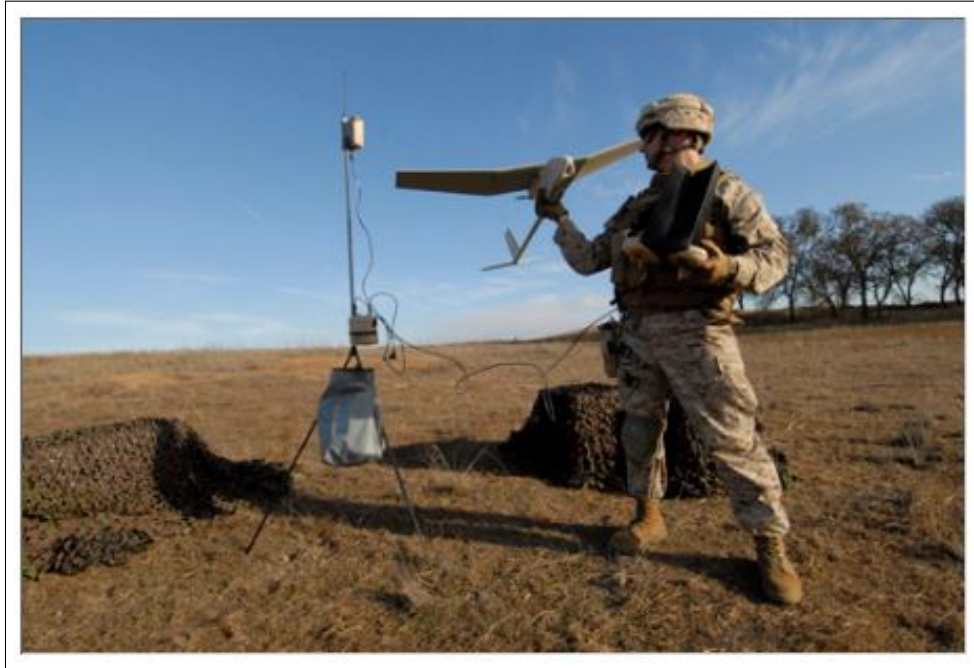
Figure 2.3: Marine preparing to hand launch the 4.2lb Raven UAV. From [8] The tripod in the back is part of Aerovironment’s Ground Control System (GCS), which “improves situational awareness of the ground, provides operators cue to potential threats, and enhances airborne intelligence, surveillance and reconnaissance (ISR)” [9].
