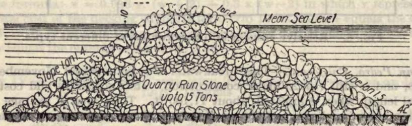
FIG. 11.—Section of Colon breakwater, Panama.
