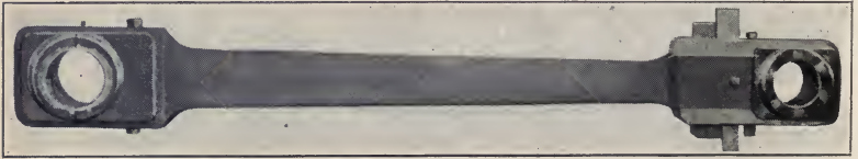
FIG. 70.—Strap end connecting rod.
