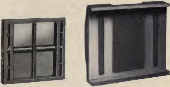
FIG. 103.—Double ported valve with cover plate.
