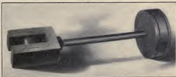
FIG. 68.—Piston, piston rod and crosshead.
