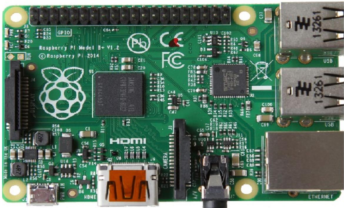
Just like you have a hard disk on normal computers, the raspberry pi has an SD card that acts as the hard disk. The OS is loaded into the SD card and plugged into the board. You can use various memory capacity SD cards: 8GB, 16GB, 32GB, etc.
