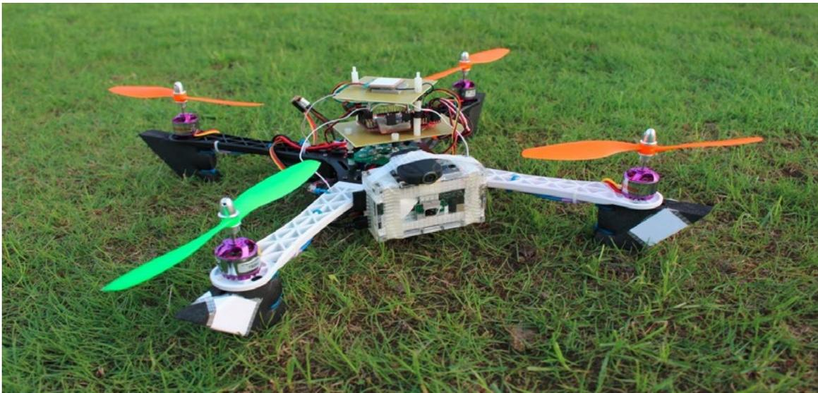
In this project, you can see a quadrotor, which has been built using a raspberry pi. The system uses IMU sensors and brushless motors for stabilizing and powering the copter.
