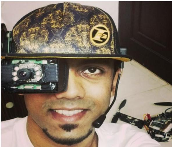
In this DIY project, I was able to create a cool head mounted display which was capable of mimicking the functions of a Google Glass, as it had: a head mounted display, voice recognition and first person video streaming using a webcam. It even got featured on Techcrunch. Check out this video:
