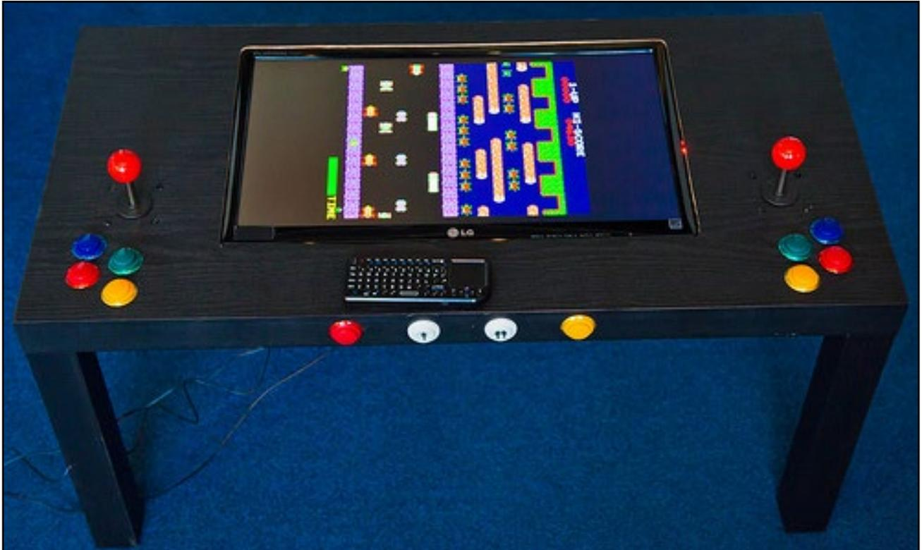
Check out this really cool application of using a raspberry pi to power an arcade gaming table. Hook up your pi to a gaming joystick and some buttons to create an arcade gaming table.
