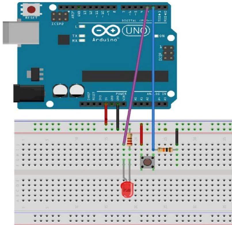
Based on the above example I will be explaining the programming structure in arduino. Here, we need to find the state of the button press and switch ON the LED accordingly. Furthermore, if the button is pressed, a HIGH (5V) voltage is passed to the digital pin; else a LOW (0V) voltage is passed.
