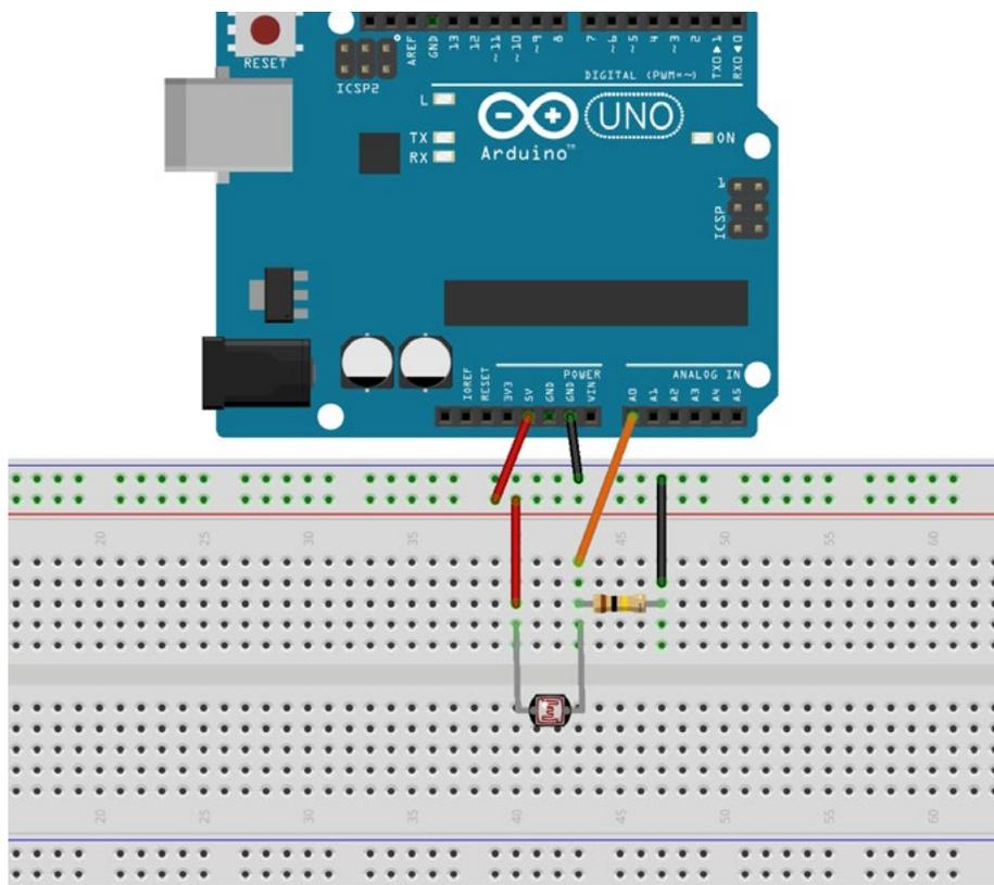
Here, one leg of the LDR is connected to VCC (5V) on the arduino, and the other to the analog pin 0 of the arduino, a 100K resistor is also connected to the same leg and grounded.
