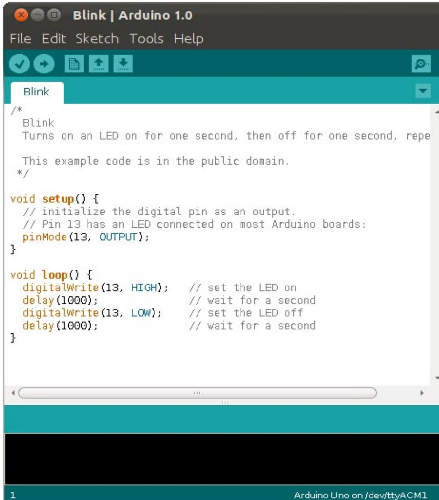
A screenshot of the Arduino IDE interface. The title bar reads "Blink | Arduino 1.0". The menu bar includes "File", "Edit", "Sketch", "Tools", and "Help". Below the menu bar is a toolbar with icons for saving, running, uploading, and downloading. The main workspace shows a sketch named "Blink" with the following code:
