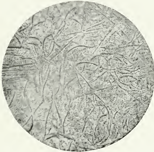
Fig. 17—Crystallites in spherulitic lava. One mile post, west boundary, Marriott township. Magnified about 40 diameters. One nicol.
