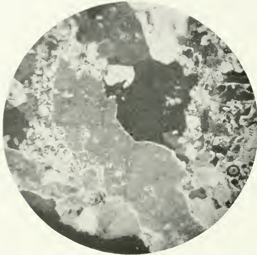
Fig. 38—Section showing granulation of primary quartz. Secondary calcite and pyrite are present. Howey-Cochenour-Willans vein, Holloway township. Magnified about 20 diameters. Cross nicols.
