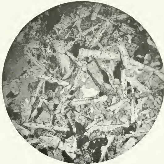
Fig. 11—Interior of basic lava flow at Howey-Cochenour-Willans gold prospect, Holloway township. Magnified about 20 diameters. One nicol. The long rods are plagioclase, the remaining parts being mostly augite and magnetite.
