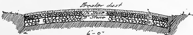
Fig. 43.—Cross section through macadam walk.—See page 48
