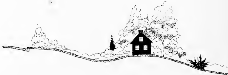
Fig. 66.—Cross section showing proper grading around a residence located on ground descending from the highway.—See page 67
