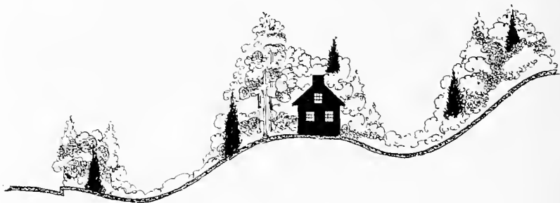
Fig. 65.—Cross section showing proper grading of portion around a residence located on ground ascending from the highway.—See page 67
