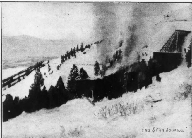
HOME-MADE SNOW PLOW COUPLED TO TWO 31-TON SHAY LOCOMOTIVES, USED BY THE EMPIRE COPPER CO.,
