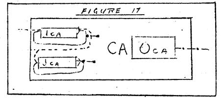
the cutside (relatively to CA, i.e. with M) by the line -.-., which conducts when a result leaves CA (for M). The circulating connections of  $O_{CA}$  and its connections with the operating parts of CA are not shown, nor the E-elements which control the connections shown (nor, of course, the operating parts of CA). (For the complete description of CA of.
