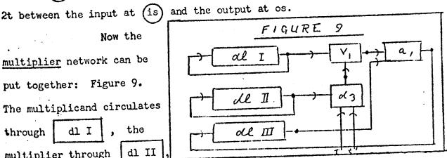
and the sum of partial products (which begins with the value 0 and is gradually built up to the complete product) through dl III. The two inputs t, t' receive the timing stimuli required by the discriminator (they correspond to t, is in Figure 8.).
