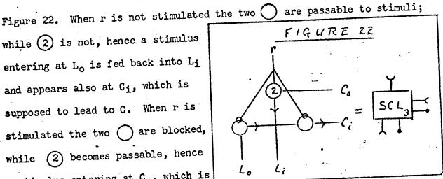
supposed to come from C, goes on to Li, and Lo is isolated from all connections. Hence SCL produces the first state of 13.3 when r is not stimulated, and the second state when r is stimulated. We also note, that in the first case a stimulus passes from Lo to Li with a delay 7 (cf. the timing question of SG1, discussed above.)
