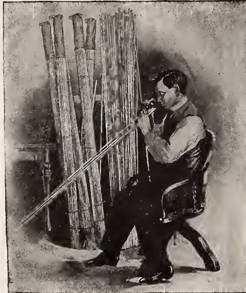
Inspecting glass tubing for Tycos Thermometers.
