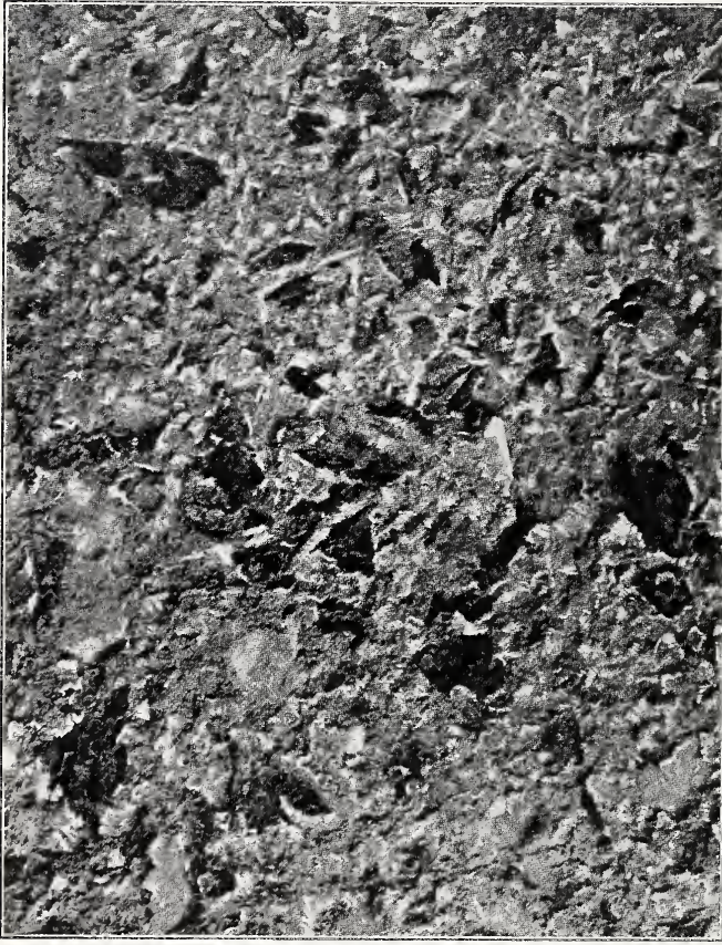
FIG. 9. SURFACE FINISHED BY HAND HAMMER OR AXE.
