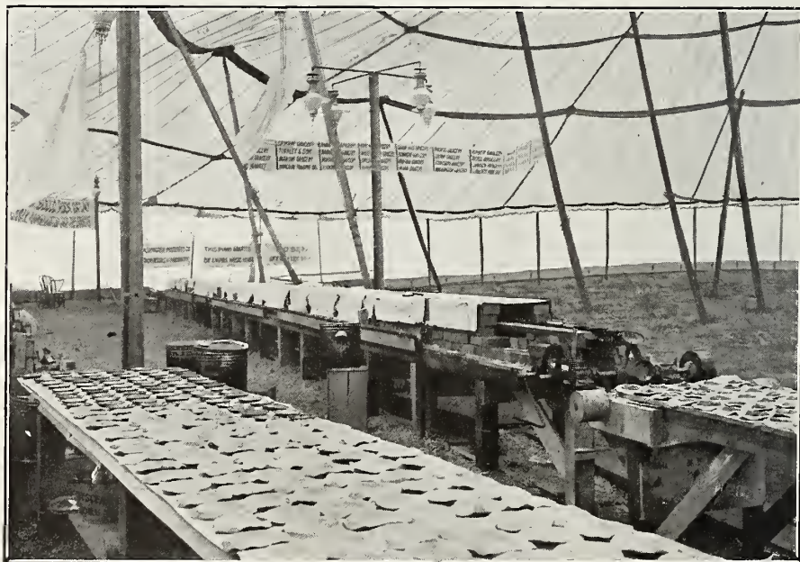
Oven seventy-five feet long, which baked fifty thousand apple pies during the National Apple Show, turning out pies at the rate of twenty-two hundred and fifty per hour. Pies were carried through on an endless chain, and were served free to the public. Fifth National Apple Show, 1912.
