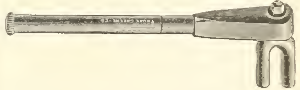
Fig. 32.—Wrench for bending and fitting the Thomas hip splint.
