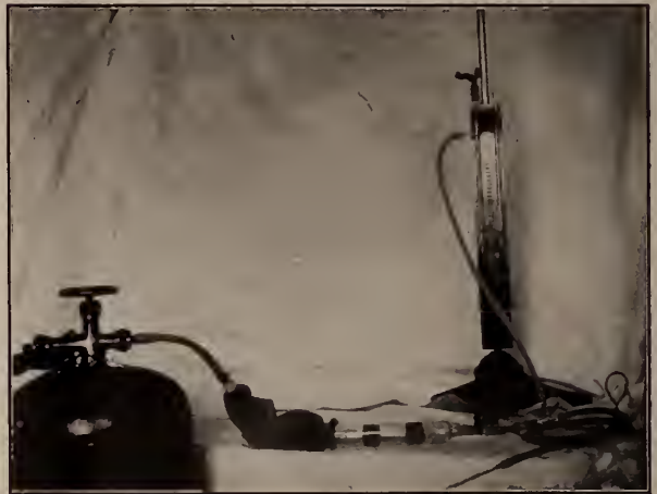
Fig. 1—Showing from left to right oxygen tank, rubber bag (400 c.c. capacity), thermometer in glass tube, water-manometer and small canula.
