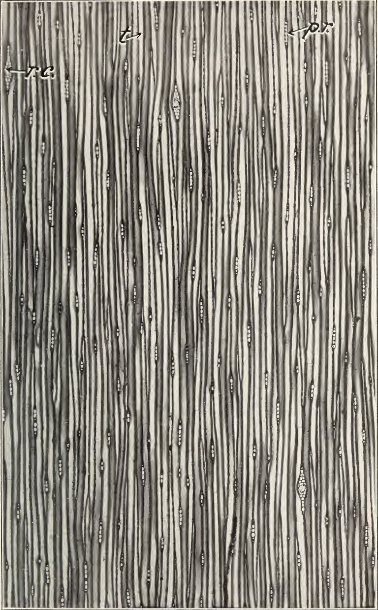
TANGENTIAL SECTION OF THE WOOD OF NORWAY PINE MAGNIFIED 50 DIAMETERS; t. , TRACHEIDS; p. r. , PITH RAYS; r. c. , RESIN CANAL IN PITH RAY.
