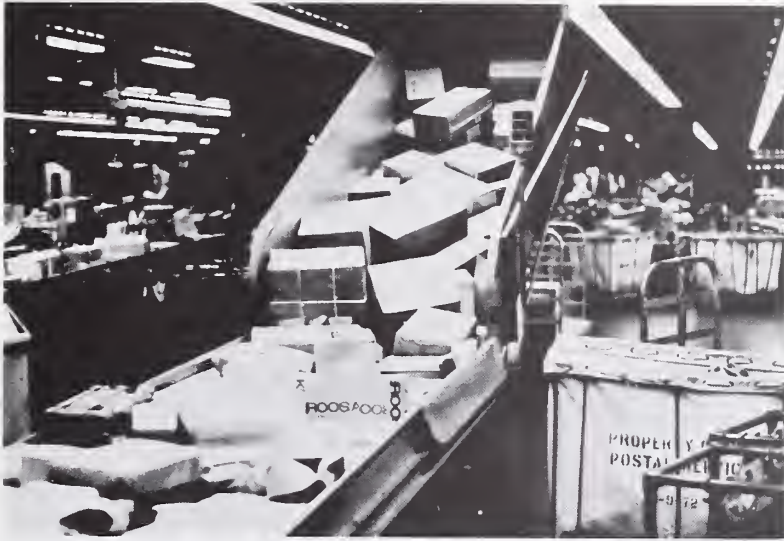
Figure 2. Conveyor--one type of postal mechanization. (NBS)
