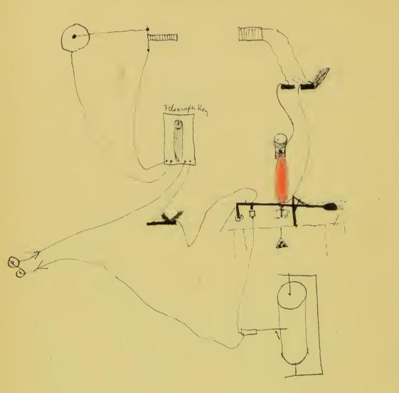
By presting on the telegraph Ray the muscle is stimulated. Toto At the same time the time monther tircuit is made. Consequence, a mark on the typicaler. But ofter a that time the muscle centrals and lifts the law. In so doing the time marker circuit is broken. Result there is another marks on the typicaler - The distance between the two marks is the latent period. It gets longer as the muscle is meighted. Ville trackings.
