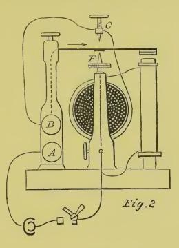
eurrent is broken; or (2) so that when the key is closed it acts as a bridge, by which so large a proportion of the current is derived, that it in effect vanishes in the part of the circuit beyond the bridge.
