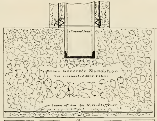
METHOD USED IN CONSTRUCTING HOLLOW EXTERIOR WALL
