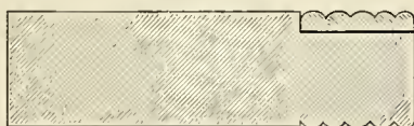
SECTION (Reduced) Of Apartment House Door Stock. Regular sizes 3 1/2 x 7/8 and 2 1/4 x 1 1/8 inches
