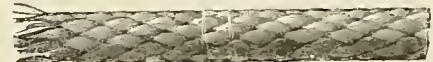
SIZE No. 10. DIAM. 5-16 In. About 44 lbs. per doz.; about 27 ft. per lb. Suitable for weights from 30 to 40 lbs. Minimum diam. of pulley allowable 2 1/2 in.
