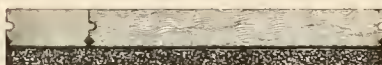
FIG. 4. SECTION OF ENGLISH WOOD BLOCK FLOOR Laid in Mastic on Concrete Foundation, Fireproof Construction
