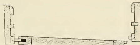
SECTION OF SLIDING SCREEN Being Spring onto the Runners
