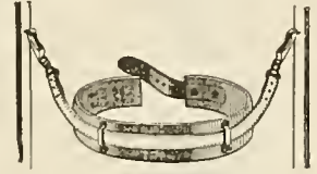
FIG. 1. SAFETY BELT WITH BOLTS IN WOOD WINDOW FRAME
