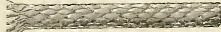
SIZE No. 9. DIAM. 9-32 In. About 33 lbs. per doz.; about 36 ft. per lb. Suitable for weights from 20 to 30 lbs. Minimum diam. of pulley allowable 2 1/4 in.
