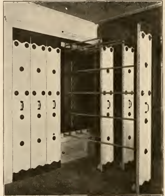
FIG. 2. DRYER SHOWING RACK SYSTEM OPERATING ON FLOOR AND ELIMINATING THE OVERHEAD TRACK SYSTEM. Rack Faces in this Type Dryer measure 11" and 12" only.
