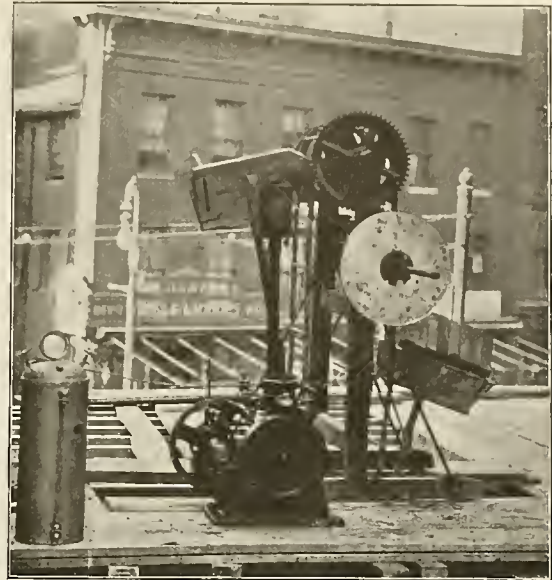
FIG. 7. THE STANLEY KEROSENE ENGINE Showing its connection to the Top of the Chain Machine
