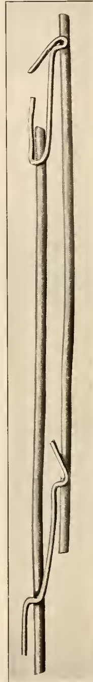
FIG. 1. ELECTRICALLY WELDED FABRIC.
