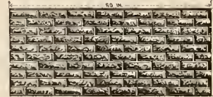
ROCK FACED BRICK SIDING
