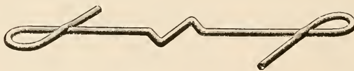
FIG. 3. MORSE PATENT WALL TIE
