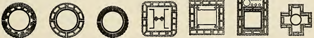
STANDARD SHAPES OF COLUMN COVERING
