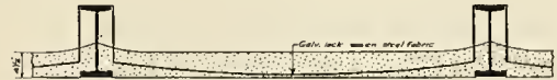
Concrete - 1 Portland cement, 2 Sand and 5 Cinders. Approved by Bureau of Buildings for 6'-0" Span with live load of 150 lbs. SYSTEM N°2 TYPE D Tested to 1500 lbs. per Sq. ft.
