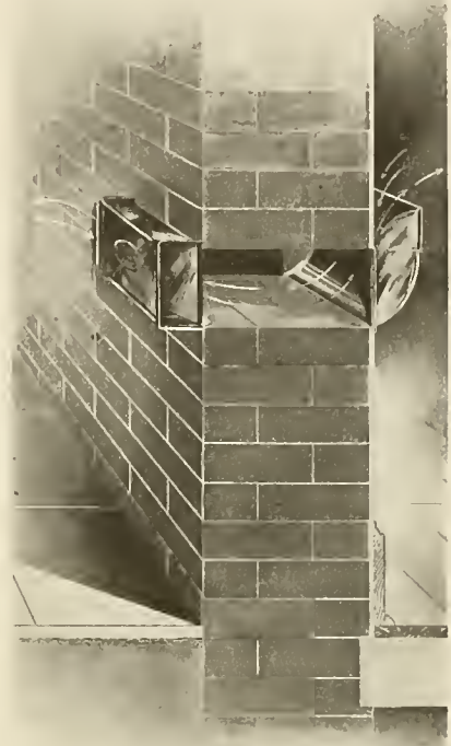
FIG. 5. MOBILE VENTILATION DEVICES INSTALLED IN WALL OF A BUILDING
