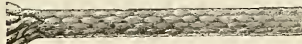
SIZE No. 7. DIAM. 7-32 In. About 22 lbs. per doz.; about 55 ft. per lb. Suitable for weights from 5 to 12 lbs. Minimum diam. of pulley allowable 1 3/4 in.
