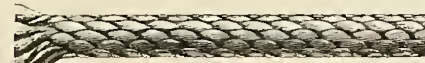
SIZE No. 8. DIAM. 1/2 In. About 27 lbs. per doz.; about 44 ft. per lb. Suitable for weights from 12 to 20 lbs. Minimum diam. of pulley allowable 2 in.
