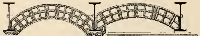
Showing Plastering on Arches Showing Use of Metal Lath Ceiling SECTION OF TYPICAL ARCHES.
