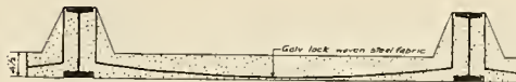
Concrete - 1 Portland cement, 2 Sand and 5 Cinders. Approved by Bureau of Buildings for 6'-0" Span with live load of 150 lbs. SYSTEM N°2 TYPE B Tested to 1500 lbs. per Sq. ft.
