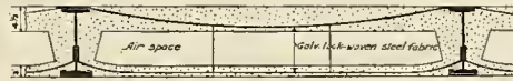
Concrete - 1 Portland cement, 2 Sand and 5 Cinders. Approved by Bureau of Buildings for 6'-0" Span with live load of 150 lbs. SYSTEM N°1 TYPE B Tested to 1500 lbs. per Sq. ft.
