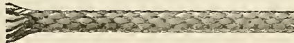
SIZE No. 6. DIAM. 3-16 In. About 18 lbs. per doz.; about 66 ft. per lb. Suitable for weights of less than 5 lbs. Minimum diam. of pulley allowable 1 1/2 in.
