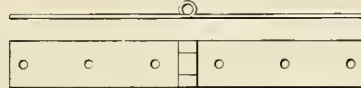
FIG. 5. CENTER HINGES Which join the two sections of the door, and allow lower section thereof to lap in under top half when door is opened
