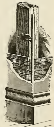
FIG. 8. APPLICATION OF PRESCOTT CORNER BEAD
