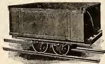
Fig. 5179. Charging Car for Boiler rooms, made entirely of steel, built with one or two doors, which can be placed either at the side or the end, or with rotary box; capacity from 500 lbs. to 2 tons of coal; gauge generally 20, 21 1/2 and 24 inches
