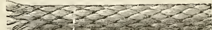
SIZE No. 12. DIAM. 3/4 In. About 60 lbs. per doz.; about 20 ft. per lb. Suitable for weights from 40 to 50 lbs. Minimum diam. of pulley allowable 3 in. The number indicates the diameter in 32ds of an inch.
