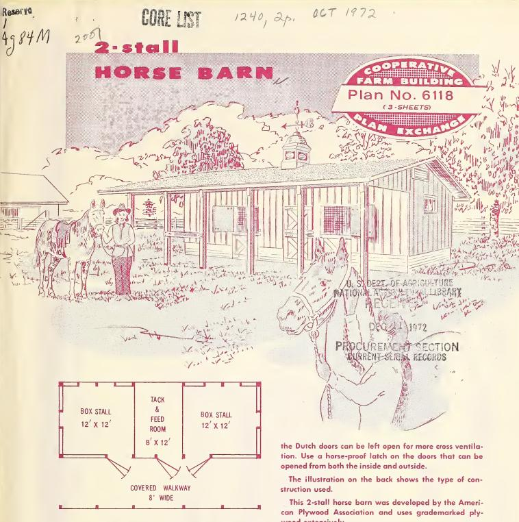
Comfortable quarters for two horses are provided by this 20- by 32-foot barn. The 12- by 12-foot box stalls, as well as the combination feed and tack room, open into an 8-foot-wide covered walkway. The use of a cupola-type ridge vent and textured one-eleven siding gives a pleasing appearance. Dutch doors provide entry to the stalls and feed room.
