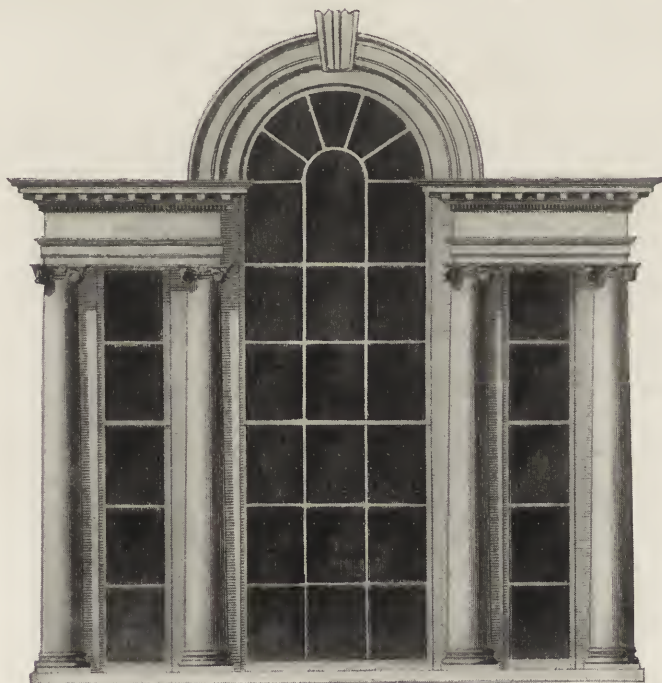
DRAWING OF VENETIAN (PALLADIAN) WINDOW FROM "THE YOUNG CARPENTERS' ASSISTANT," BY OWEN BIDDLE, PUBLISHED IN PHILADELPHIA, 1805.
