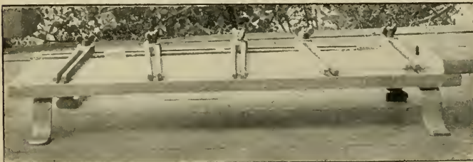
Fig. 1.—Smith's foundation-cutter, with movable guides that may be set for any size of starter desired.
