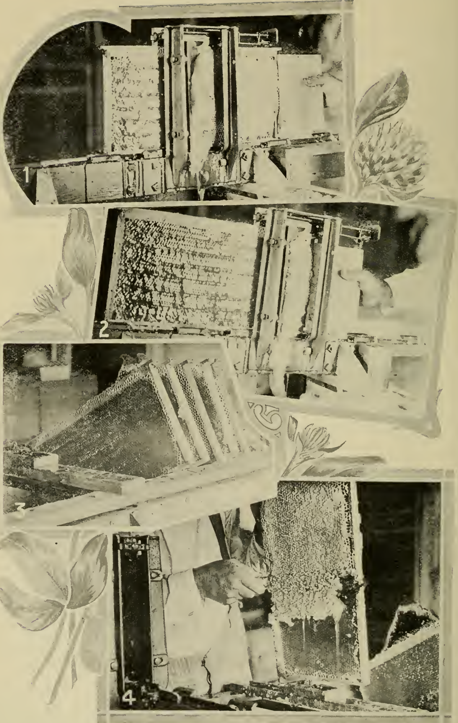
UNCAPPING COMBS IN A FERGUSON UNCAPPING-MACHINE AND BY HAND. An inexperienced man can do as much with the machine as an expert can with the ordinary hand-knife.
