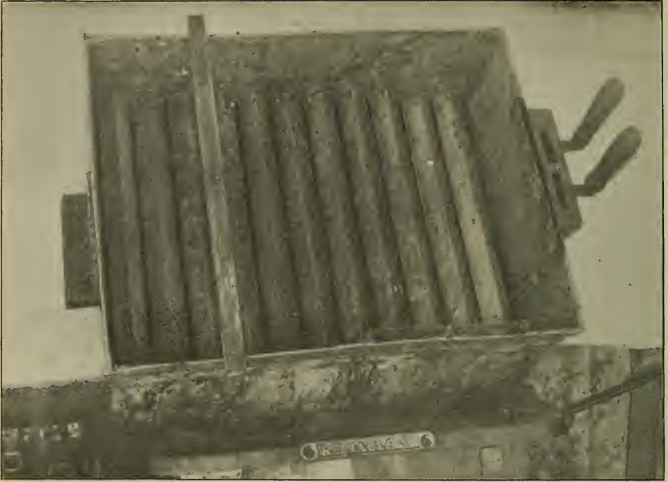
F. J. Severin's capping-melter, showing the melting surface made of square tubes, the metal scraper for the knives, and the slots for heating them.
