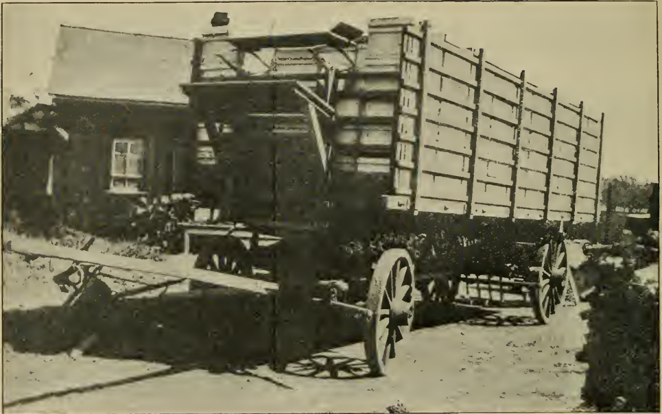
Fig. 3.—Rack made in California especially for hauling bees.
