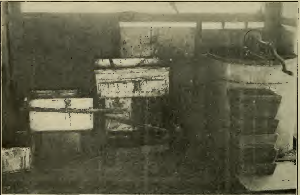
FIG. 2.—Interior of F. J. Severin's honey-room, showing extractor, capping-melter, and wax-separator.
