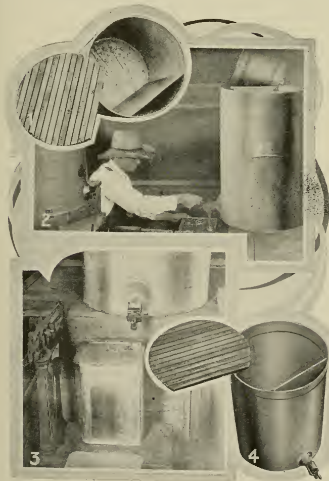
E. D. TOWNSEND'S LATEST SEPARATING-TANK FOR CLARIFYING HONEY WITHOUT A STRAINER.
