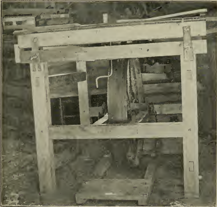
Fig. 1.—Cut-off saw-table for cutting bee-keepers' supplies; built by Percy Orton.
