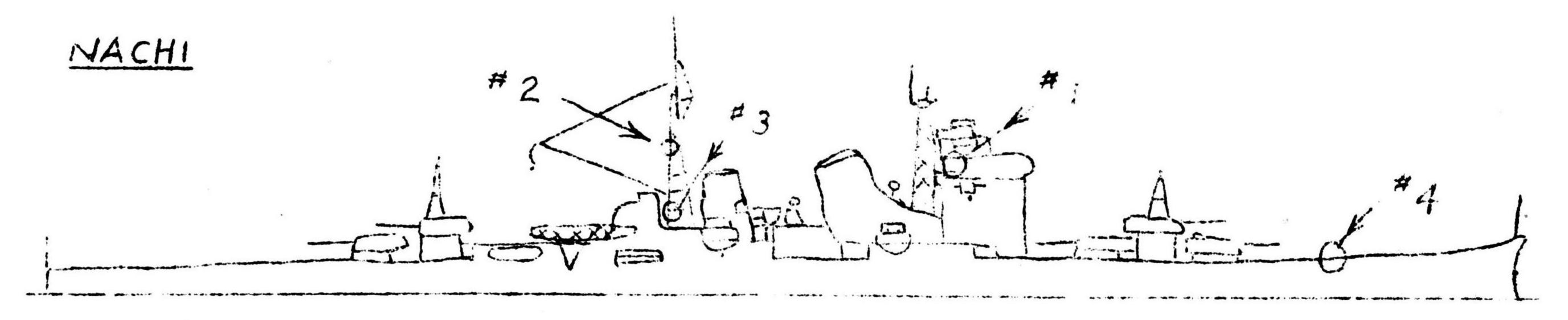
HIT #1, O+ 5 TO 10 MIN., 6 IN., BLUE DYE, S+B'D. TO PORT, KILLED 3 COMMUNICATION
