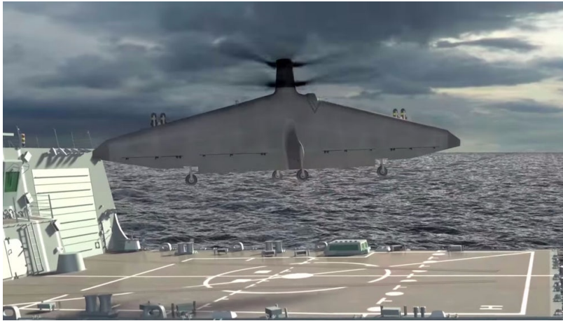
Artist's rendition of a Tern taking off from a ship's helicopter pad.
