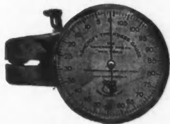
The Ashcroft Thickness Gauge
