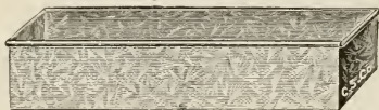
Fig. 12.—Galvanized tray or tank to be used with the support for tubes in showing capillary rise of water. Also useful for exercise No. 17
