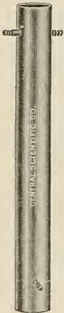
FIG. 13.—Percolation soil tube. In comparing the percolation of water through several soils the tubes are placed in the support block (Fig. 14) and are connected by rubber tubing attached to the lateral inlets. A beaker is placed under each drainage tube.
