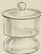
FIG. 9.—Moisture-proof chamber for use in cooling oven-dried samples before weighing. Moisture-absorbing chemicals, as strong sulfuric acid, may be placed in the lower part to insure dryness.
