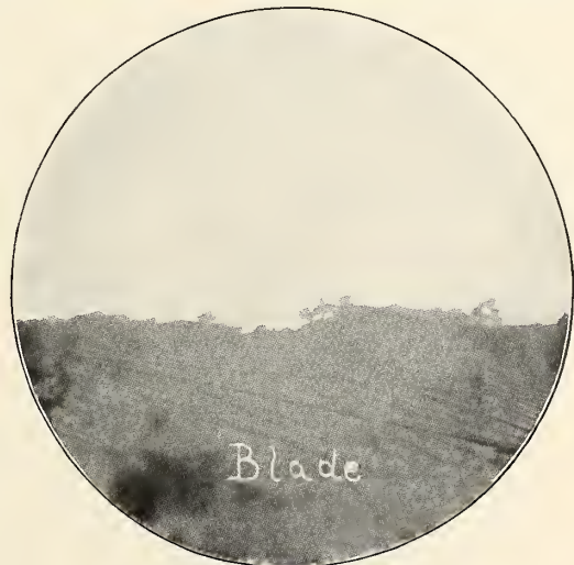
THE EDGE OF A NEWLY-HONED RAZOR-BLADE. (Greatly Magnified.)
