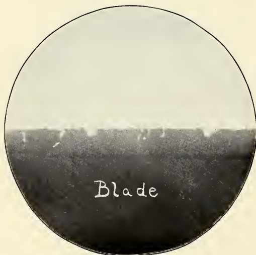
A "WIRE EDGE" ON A POCKET-KNIFE.
