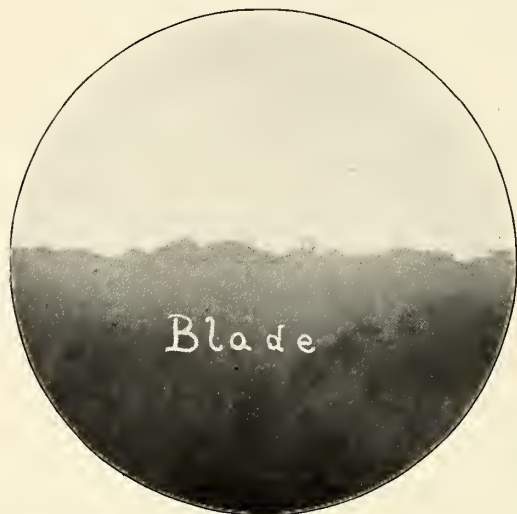
A PROPERLY SHARPENED PEN-KNIFE.
