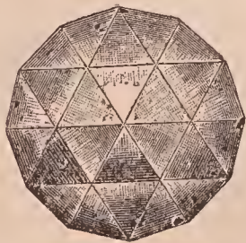
Diagram Showing the Facets of a Rose-diamond.
