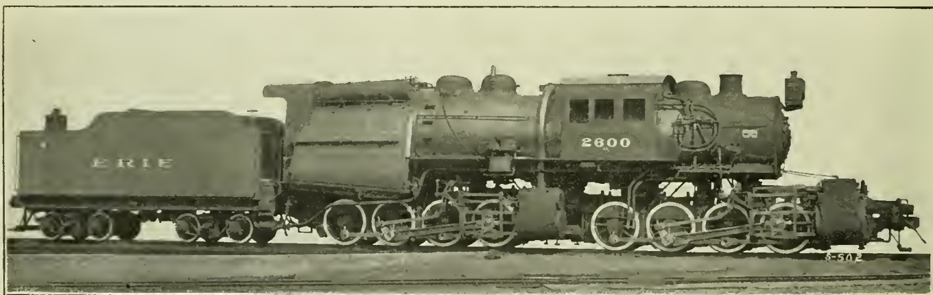
FIG. 1.—MALLET ARTICULATED COMPOUND LOCOMOTIVE OF THE TYPE TESTED ON THE ERIE RAILROAD.
