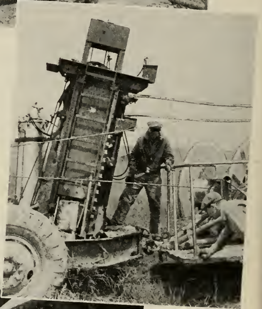
FIG. 23, above: Loading a reel of cable onto a trailer. The yoke is being pulled up by a line from a multi-drum tractor winch, and the latches will catch the spindle after another foot of travel. FIG. 24, right: The share of the cable-laying plow is in its upper position, so that the cable can be fed through it at the start of a laying operation. FIG. 25, below: This is how twin cables feed out through the foot of the plow share and are pulled through and staked before the train moves ahead
