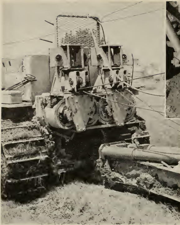
FIG. 19, left: A multi-drum winch on a tractor. It is used for adjusting the depth of the plow, loading cable reels, and moving trailers. FIG. 20, above: This relay winch pulls the tongue end of the rear trailer into a special keeper which serves as a coupling. Paying out the wire rope permits the trailer to drop behind
