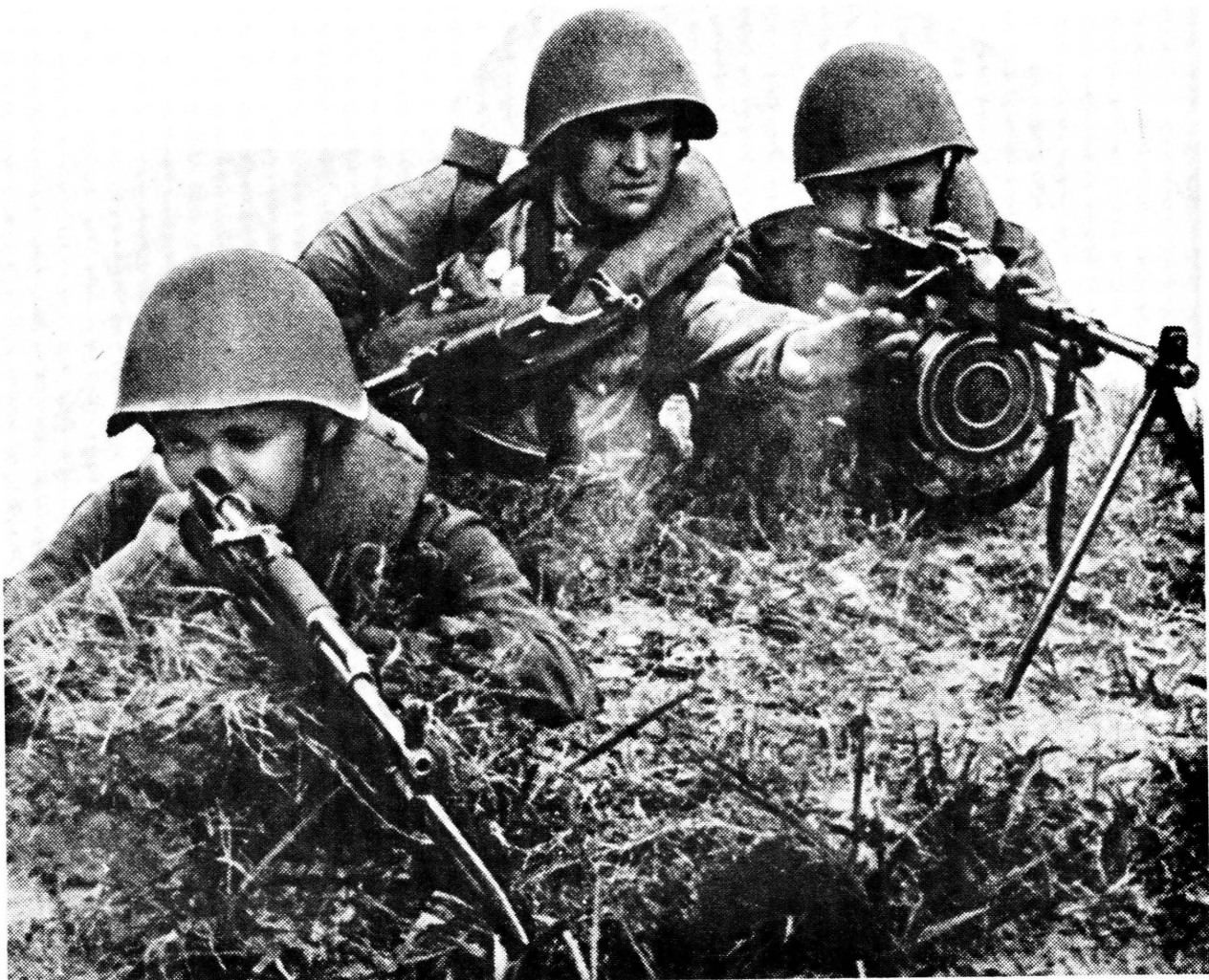
Figure 63. Soviet 7.62-mm Rifle Squad Weapons: (Left) SKS Semiautomatic Carbine. (Center) AK Submachinegun. (Right) RPD Light Machinegun.
