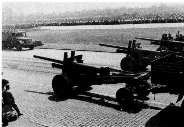
Figure 82. Soviet 122-mm Field Gun M31/37 (A19) (here shown in a Czechoslovak parade).
