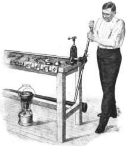
FIG. 16.—Threading wrought pipe—after one or two threads are cut, pushing is unnecessary and the operator may turn the stock as above indicated
