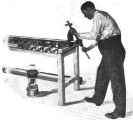
FIG. 15.—Threading wrought pipe—position of the operator when pushing the stock and die to start the thread
