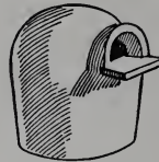
FIG. 2.—Covered pot for glass melting, as used for flint glass and optical glass.
