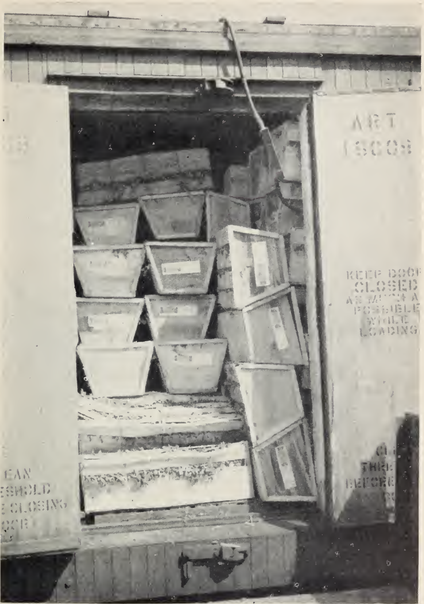
FIGURE 20.—Appearance of test shipment of tomato plants at destination when crates had been improperly stacked during loading.
