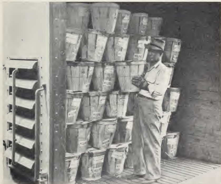
FIGURE 6.—Hampers of tomato plants are stacked in refrigerator cars for shipment. For proper cooling they should not be stacked higher than the bottom of the top opening of the end bunkers. This load is one layer higher than is advisable.
