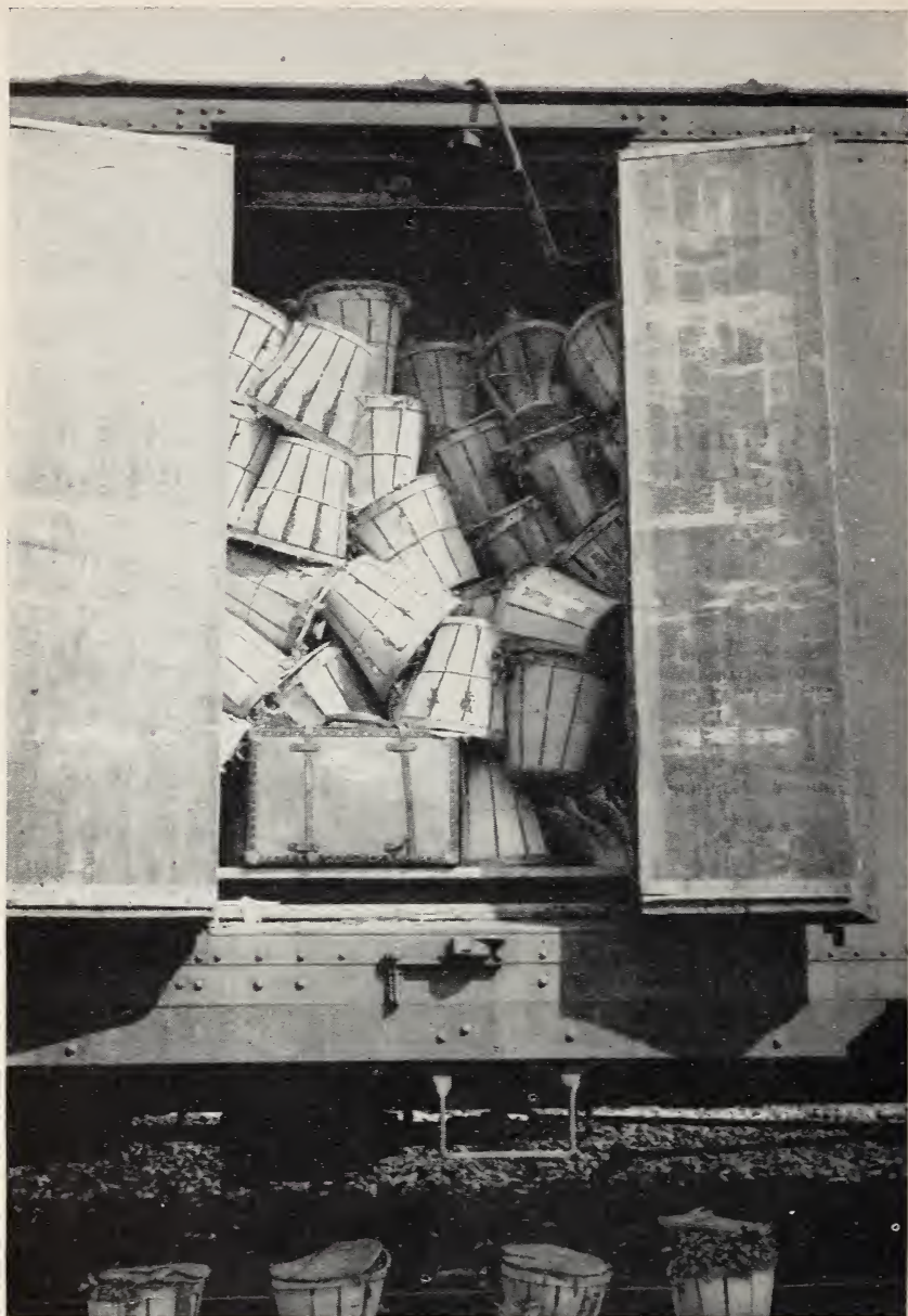
FIGURE 19.—Appearance of test shipment of tomato plants at destination when hampers had been improperly stacked during loading. Hampers beneath car fell out when doors were opened. Suitcase in doorway was for temperature equipment seen at top of doorway.
