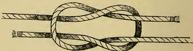
Thief Knot —Worthless, will slip; notice ends on opposite sides.
