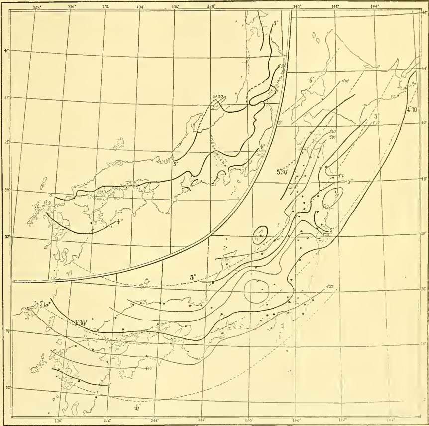
MAP OF JAPAN SHOWING THE LINES OF EQUAL MAGNETIC DECLINATION. (ACCORDING TO KNOTT AND NAUMANN.)
