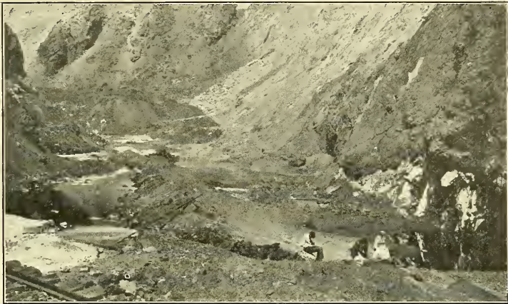
FIG. 1. Open cut workings at Isabella, Tennessee, showing light-colored deposit of Pisanite above water in the lower right hand corner.
