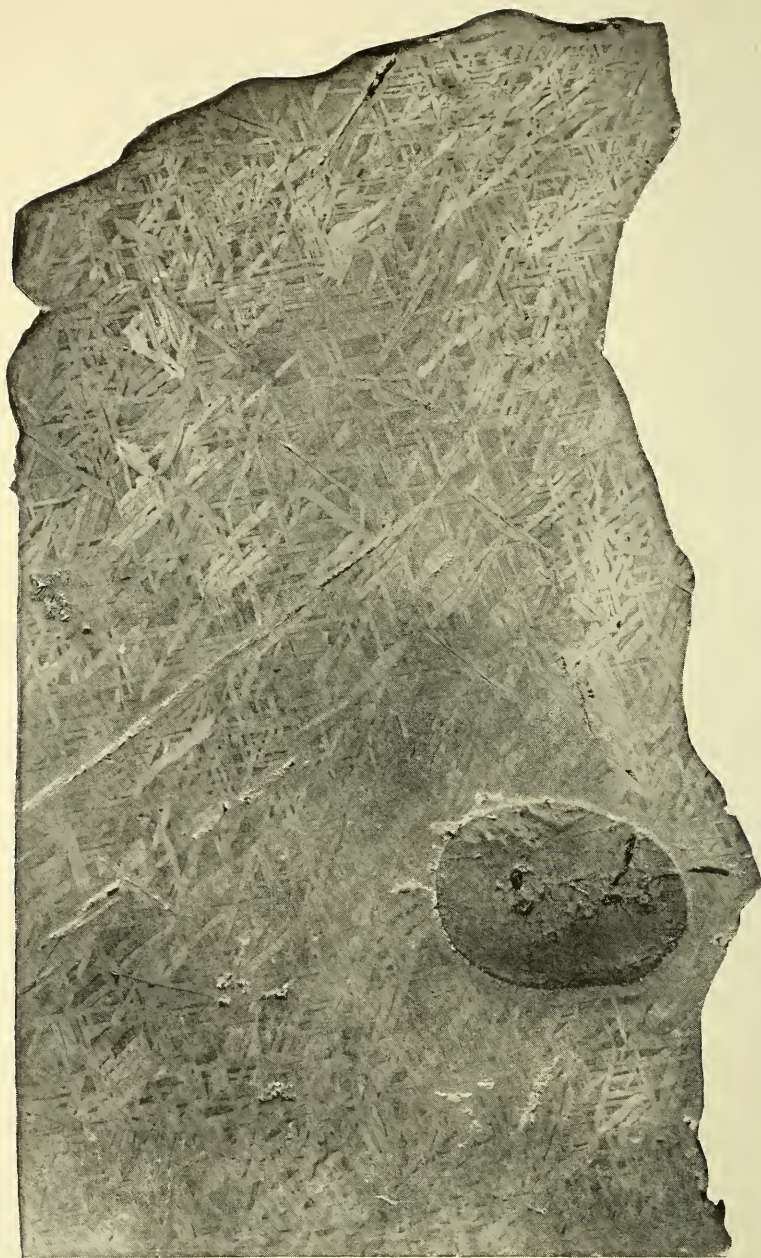
FIG. 5. Showing kamacite and plessite.
