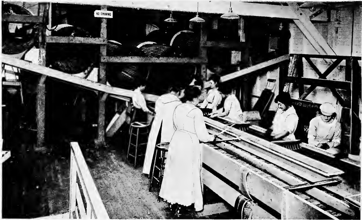
A SECOND CULLING OF THE MACHINE-GRADED NUTS BY HAND, FURTHER GUARANTEES THEIR QUALITY
