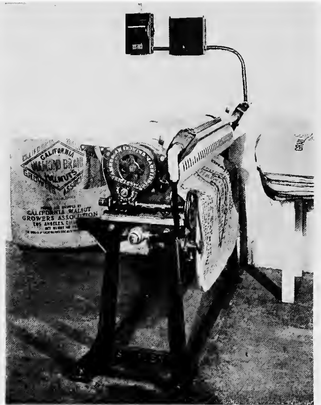
"THE MANGLE," A SPECIAL MACHINE RECENTLY INSTALLED IN THE LOS ANGELES HEADQUARTERS OF THE ASSOCIATION, IN AN ATTEMPT TO PREVENT THE SPREAD OF THE CODLIN MOTH THROUGHOUT THE STATE. SIXTY THOUSAND EMPTY DIAMOND BRAND WALNUT BAGS ARE BEING "IRONED OUT" BY THIS MACHINE THIS SEASON, THE IDEA BEING TO EXTERMINATE THE INSECTS BY HEAT AND PRESSURE
