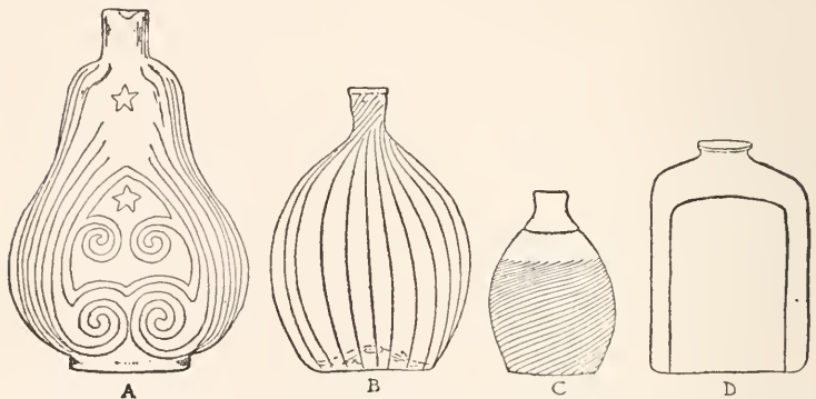
Fig. 1. Old American Bottles: A, fiddle-shaped, raised design of stars and scrolls; B, ribbed or corrugated sides; C, spiral ribbed or corrugated sides, from Pitkin Glass Works, Manchester, Conn., between 1783 and 1830, blown in patterned moulds; D, square-shouldered snuff bottle, made at Coventry, Conn., c. 1825.
