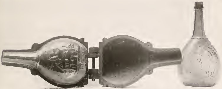
1 and 2, "Green" Glass Saucer and Milk Bowl, New Jersey, Early Eighteenth Century 3-7, Tumblers, Wine Glasses and Milk Bowl, Eighteenth and Early Nineteenth Centuries Courtesy of Pennsylvania Museum and School of Industrial Art 8 and 9, Bottle Mould and Moulded Bottle, Early Nineteenth Century Courtesy of Pennsylvania Museum and School of Industrial Art
