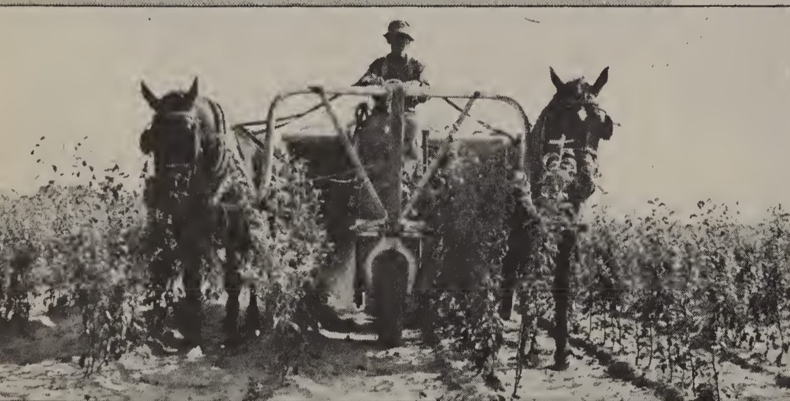
Spraying a field of 200,000 one-year apple trees. This Emlong-designed machine soaks them from all directions, even after six feet tall.
