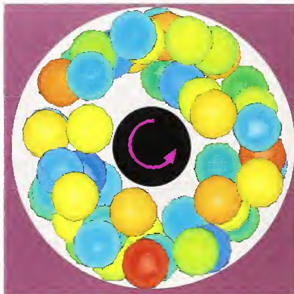
Fig. 11. Coaxial Rheometer. An inner cylinder (in black) subject to an applied torque rotates, causing the motion of the spheres.
