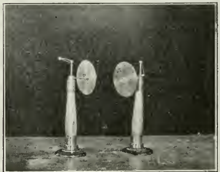
FIG. 12.—Two brass plates on glass stands. Plates separated. One plate charged, as shown by the repulsion of the pith-ball.
