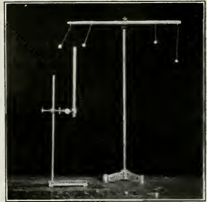
FIG. 8.—Negative ebonite rod between two balls, left charged negatively from ebonite rubbed with cat's fur, the other charged positively from glass rubbed with silk. Like charges repel, unlike charges attract.
