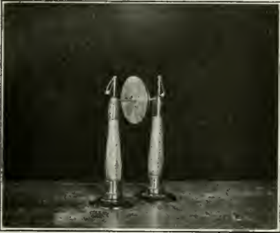
FIG. 13.—The same plate as in figure 12 (with the same charge) after plates were placed close together, but not touching. Note that the pith-ball has dropped showing less repulsion. More electricity can now be given to the charged plate. That is why the plates when close together are called a "condenser."
