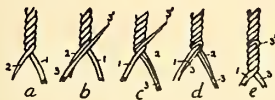
FIGURE 13.—Two-ply cord, joining ply ( so'o ): a, the ply (2) is the shortening ply; b, the new strand (3) is directly laid over the short ply (2) from below with its short end (3') projecting upwards past the point of joining; c, the other ply (1) is twisted around over the reinforced ply (2); d, the projecting upper short end (3') is doubled down over the other ply (1); e, the twisting is carried on and both the short end (3') of the new strand, and the short ply (2) is buried so to speak in the twists, while the new strand (3) continues the ply (2).
