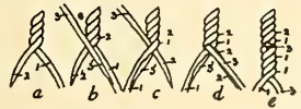
FIGURE 14.—Two-ply cord, alternate join: a, the alternative method is exactly the same in result but the opposite in commencement technique. The ply (2) is again the shortening ply; b, the new strand (3) is added from above with its short end (3') on the long ply (1); c, the ply (1) with the short end (3') is twisted over the short ply (2); d, the long end of the new strand (3) is doubled down over the short strand (2); e, the twisting is carried on with the same results as in figure 125.
