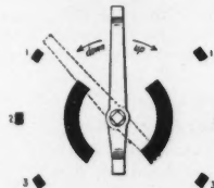
Fig. 18. Sketch of the Switch in the Elevator with which the Operator Controls the Car.
