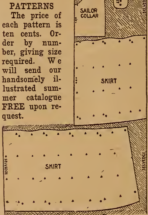
How the Pieces of the Pattern Are Placed on Material a Yard Wide
