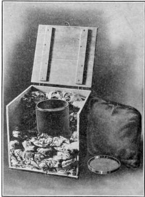
FIG. 4.—Homemade fireless cooker with part of outside container removed to show packing of crumpled paper and the cooking vessel, with its container.
