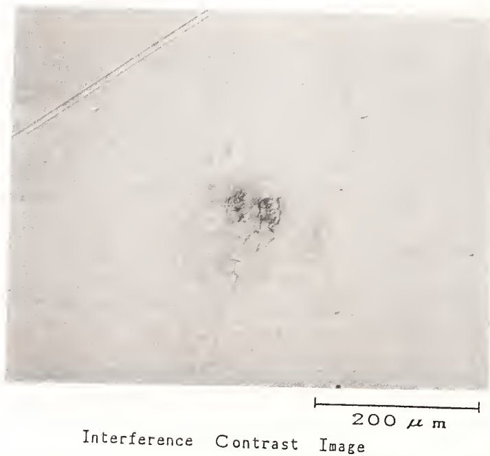
Figure 12. Damaged microstructure of the e.b.m. Mo mirror surface after the repetitive irradiations of 26 shots.
