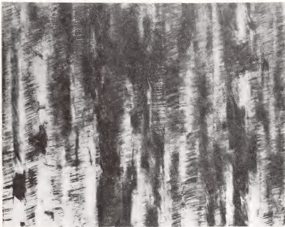
Figure 3 Microstructure of alloyed ZnS_xSe_{1-x} film on glass substrate
