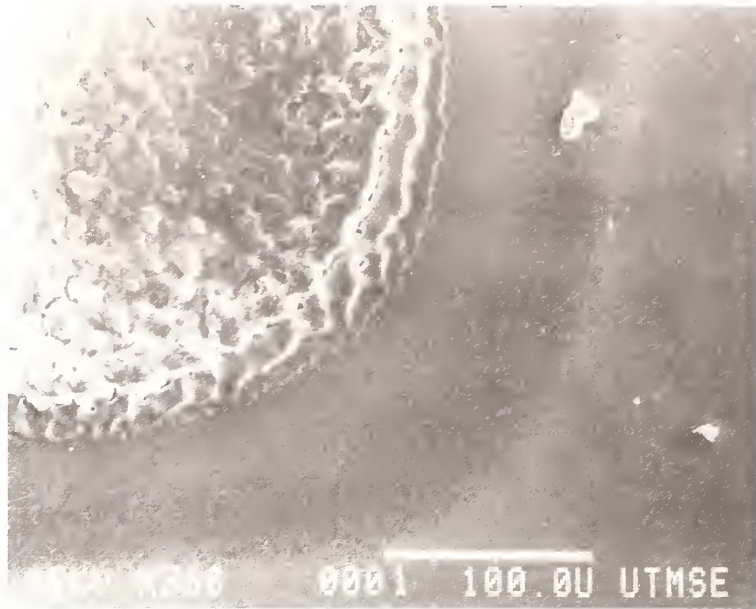
Figure 9. SEM micrograph of damage due to 30 pulses at an average fluence of 0.38 \text{ J/cm}^2 .
