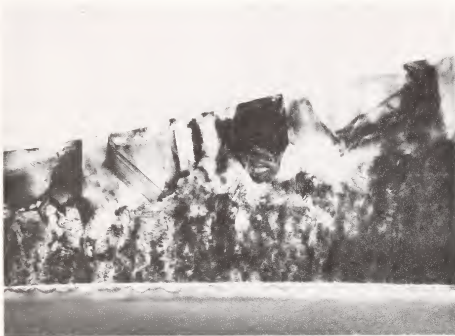
Figure 7 Cross sectional TEM image taken of ZnS film at periphery of laser damage site. Degree of melt back of ZnS induced by heating effect of laser driven plasma is clearly shown
